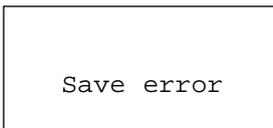
While storing items in the directory, the cordless handset has lost communication with the base unit. Move closer to the base unit and try again.
