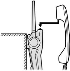
To temporarily set the handset down during a conversation, place it as shown here.
