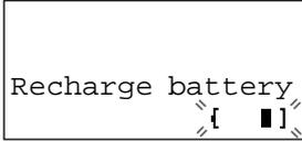
The battery needs to be charged. Place the cordless handset on the charger to charge the battery (p. 12).
