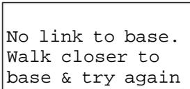
The cordless handset has lost communication with the base unit. Move closer to the base unit and try again.
