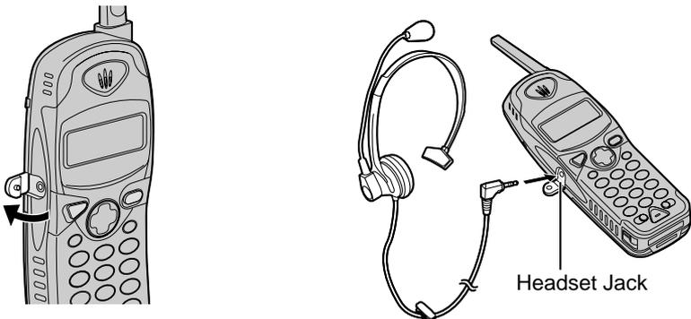
When the optional headset is connected to the cordless handset, make sure to use the headset to talk with the caller. If you want to have a normal cordless phone conversation, disconnect the headset.
