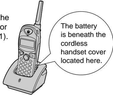
The battery is beneath the cordless handset cover located here.
