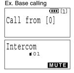
To end the intercom, press **OFF** or place the handset on the base unit or the charger.
