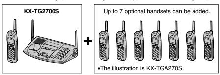
The included handset is pre-registered at the factory and assigned the extension number 1. You do not need to register this handset which has "[1]" on the display.
