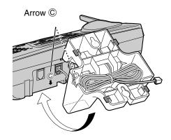
While keeping the adaptor held to the base unit, slide the wall mounting adaptor to the left until it clicks into place.
