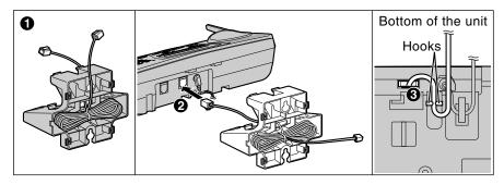
Insert (A) and (B) hooks on the wall mounting adaptor into the holes on the base unit.
