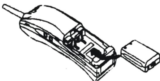
3. Place the cover and slide the cover up until it latches into the handset.
