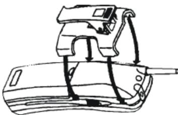
3. Press firmly until the belt clip snaps into place.
