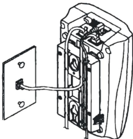
6. Place the base station on the posts of the wall plate and push down until it is firmly seated.
