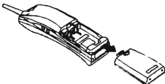
2. Slide the battery down into the handset.
