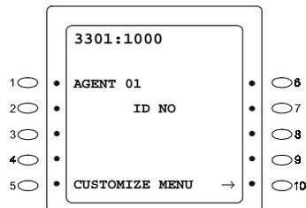
4. Enter 4-digit ID number using the 10-key pad. (The figure on left shows setting of Agent No.01.) To clear ID press **CONF** key.
