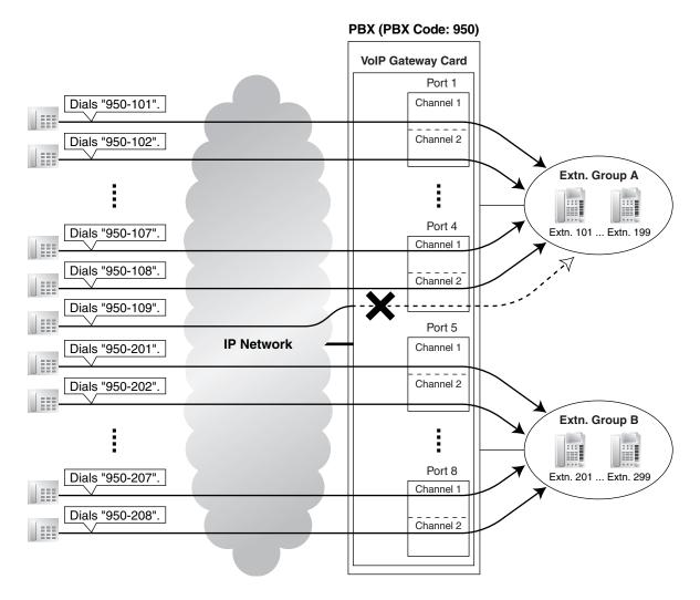
It is possible to program the PBX to allocate separate groups of VoIP gateway ports to individual extension groups A and B for making outgoing calls. With this programming, each extension group, A and B, can have a group of ports for its exclusive use.
