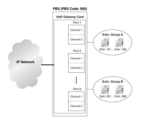
Hunt pattern programming determines the VoIP gateway ports through which to route incoming calls, depending on the received numbers. The following examples provide 2 different methods of hunt pattern programming.
