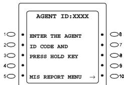
3. The following screen appears. Enter the 4-digit ID code of the target agent by using the **10**-key pad.
