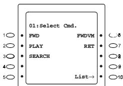
1. Press the **soft** keys **1, 2, 3, 6** or **7** for the commands to be set, and press the **HOLD** key.
