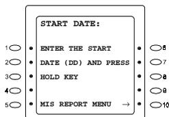
5. The following screen appears. Enter the starting date and ending date of the data to be output. First enter the starting date, press **HOLD** key to validate, then enter the ending date and press **HOLD** key again. No month is needed to be entered. For example, data for a period beginning with April 25 and ending with May 2, Enter 25 as the starting date, 2 as the ending date. For 1 through 9, 01 through 09 can be entered instead.
