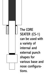
Type -S dies are 1-inch in diameter, with a 5/8-24 shank, and fit into the ram of the Corbin CSP-1 All-Steel press. The type -M dies are 3/4-inch in diameter, with a 5/8-24 shank, and fit into the ram of the CSP-1 or the CSP-3 Silver Press (horizontal). The 3-die set consists of a CORE SWAGE (CSW-1), a CORE SEAT(CS-1), and a POINT FORM (PF-1) die, each with one internal and one external punch.
