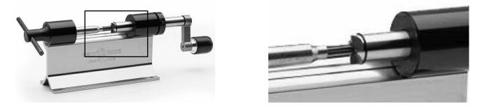
The Forster Neck Reamer will remove excess brass from the inside neck walls of cartridge cases. High-grade tool steel and a staggered-tooth design enable the Forster Neck Reamer to cut brass smoothly without chatter. Forster Neck Reamers are ground .0025"-.003" larger than maximum bullet diameter, therefore **neck reaming should be done after the case has been fired with a full load and before the neck or full length sizing operation.**
