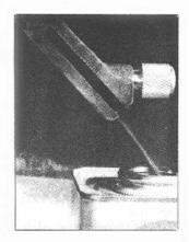
It is not necessary to remove your Forster Bench Rest<sup>®</sup> Measure from the bench in order to empty the hopper. Lift the handle 90°, remove the metering rod, set the powder can under the opening, and lower the handle. Every kernel will drain from the hopper.
