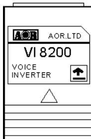
The legend "VOICE INVERT" confirms selection of the voice inverter menu. PUSH the key to toggle the voice inverter on/off (default **on**). Use the main dial or  $\uparrow \downarrow$  keys to make selection of tone in 157 steps from 0 to 156, the  $\leftarrow \rightarrow$  keys are used to increment selection by 10.
