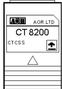
Insert the CT8200 slot card and switch the AR8200 on, select VFO mode.
