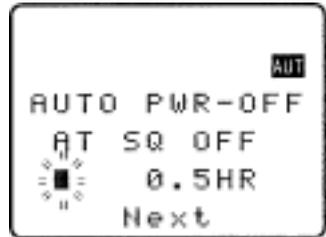
When the AR8200 squelch closes, the CPU will wait the length of time programmed in auto-power-off before automatically switching the AR8200 off. If the squelch opens again before auto switch off time has elapsed, the radio will not power down and the counter will be reset (i.e. an open squelch defeats auto power off).
