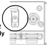
The d.c. input socket uses a mini 2.1mm power connector. This connector is configured CENTRE POSITIVE, the chassis of the receiver is at negative ground. If a power supply has been provided with the AR8600 (depending upon world market area), it is pre-wired and provides a nominal 12V d.c. output with suitable connectors being fitted as standard for the a.c. power input and connection to the AR8600.
