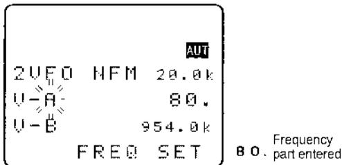
If keying in a whole MHz such as 118.000 MHz there is no need to key in either the decimal point or trailing zeros, they are all added by the AR8600 microprocessor.
