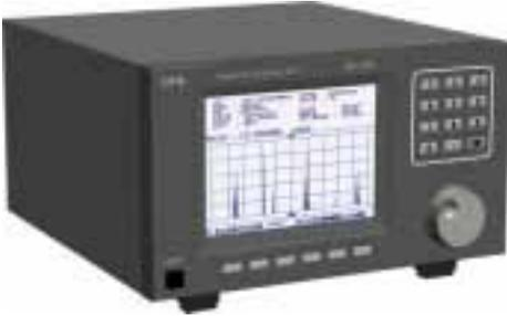
The SDU5500 provides an excellent tool for locating elusive transmission with a PEAK capability to 'freeze' the briefest of transmissions for later measurement of frequency and level after the event. A free supporting PC software package provides a virtual on-screen display of the SDU5500 with AVI video recording to disk so that events may be replaced at varying speeds for historic analysis.
