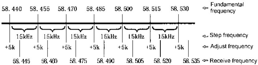
With the above in mind, 58.445 MHz with 15 kHz steps in mind, while in VFO mode, key in the start frequency of 58.445 MHz
