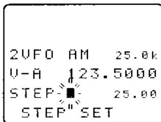
The bottom line of the LCD displays the legend "STEP SET" to indicate that the AR8600 is inviting you to change the step size.
