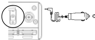
The tip on the cigar plug must be positive (+), the vehicle must be negative ground. A 1A fuse should be fitted inside the cigar lead, should this fuse blow for some reason, ensure it is replaced with the correct type. Avoid short circuits.
