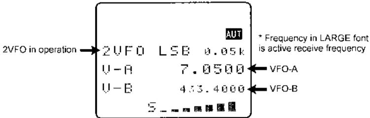
**PUSH** the **2VFO** key to first select '**VFO mode**' (should the receiver be scanning or searching etc). Each time the **2VFO** key is pushed VFO "**V-A**" and VFO "**V-B**" alternate between active and standby.
