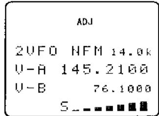
Step-adjust may be factory pre-programmed into the bandplan data (you may override this). It is also possible to store the step-adjust data into memory channels and search banks.
