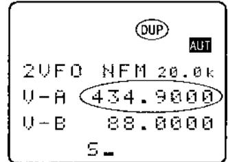
**Note:** Each VFO, memory channel and search bank can be programmed with a different frequency offset. If different channels and offsets have been programmed to VFOs etc, the key sequence  $\text{FJSHG}$  **FLJNC**  $\text{FJSHG}$  **Aa** will recall the specific offset location originally used during programming, this is particularly useful when you simply wish to toggle the + / - offset.
