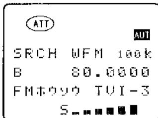
To toggle the attenuator on/off **JSH** **FUNC** **JSH** **1 AK** The legend "ATT" confirms selection and incoming signals will be reduced in strength. To toggle on/off again just repeat the sequence **JSH** **FUNC** **JSH** **1 AK**, the legend "ATT" is extinguished when the attenuator is OFF.
