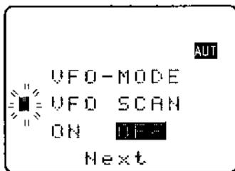
The third line displays "ON" and "OFF" with the "OFF" legend displayed in reverse contrast to show that it is currently selected (default). To toggle the VFO SCAN on/off  $\text{JSH}$  the  $\text{PASS}$  key or use the main dial or  $\leftarrow \rightarrow$  keys.
