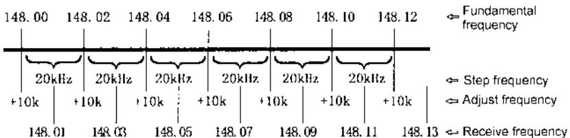
With the above example of 148.010 MHz with 20 kHz steps in mind, while in VFO mode, key in the start frequency of 148.010 MHz
