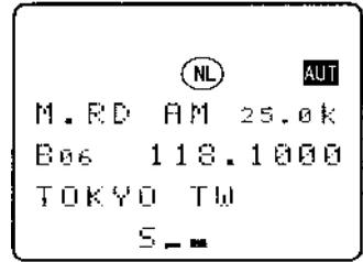
The selection of noise limiter is held separately in each VFO, each memory channel and may also be toggled during search (in scan mode, the scanning process must be stopped in order to see which memory channel you are applying the noise limiter to!).
