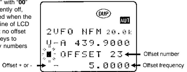
Presuming that data is already programmed into an offset location,  $\text{FJSHG}$  the **PASS** key to toggle offset between "+" positive and "-" negative offset, this is a *global toggle* and affects ALL frequency offset channels (but not those already stored into memory or search banks). To accept the offset setting,  $\text{FJSHG}$
