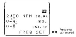
If keying in a whole MHz such as 118.000 MHz there is no need to key in either the decimal point or trailing zeros, they are all added by the AR8600 microprocessor.
