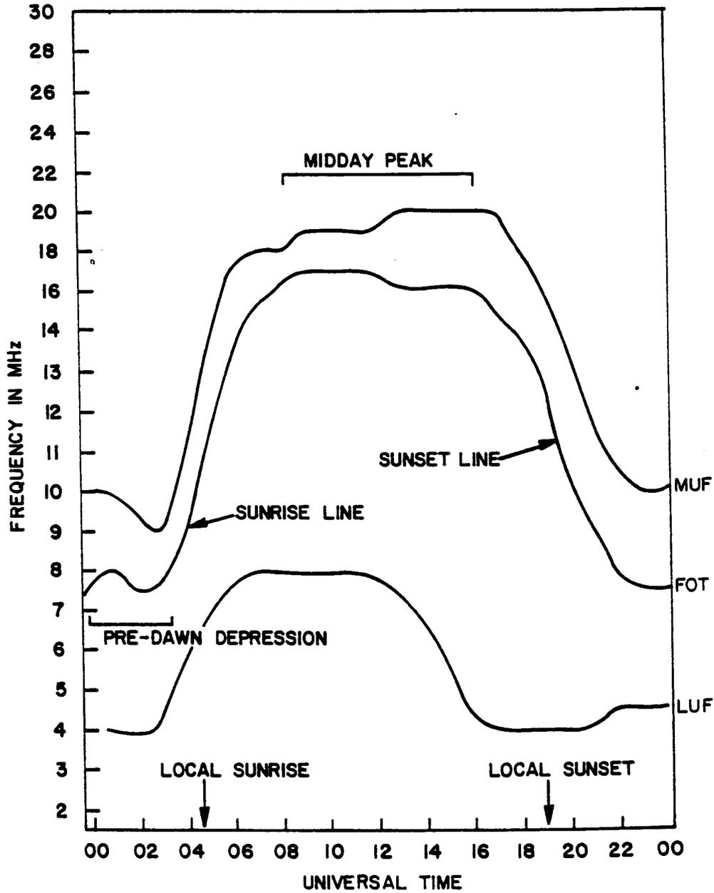
Figure 6 Important features of a typical propagation chart. (M=MUF; F=FOT; L=LUF).
