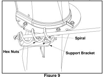
Adjust the support bracket inward or outward so that the spiral is fully engaged in the notches on the chute before retightening the hex nuts.
