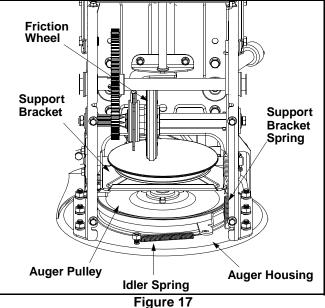
• Slip belt between friction wheel and friction wheel disc. See Figure 18. Remove and replace belt.
