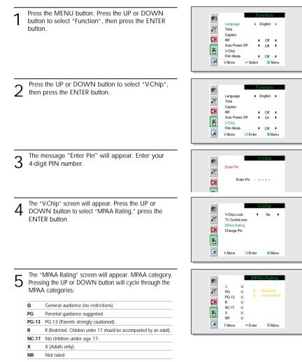
If the TV is tuned to a restricted channel, the V-Chip will block it. The screen will go blank and the following message will appear: "Excessive rating."
