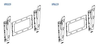
The wall mount bracket is delivered separately. Please tighten the captive screw in the direction of the arrow after assembling the bracket.
