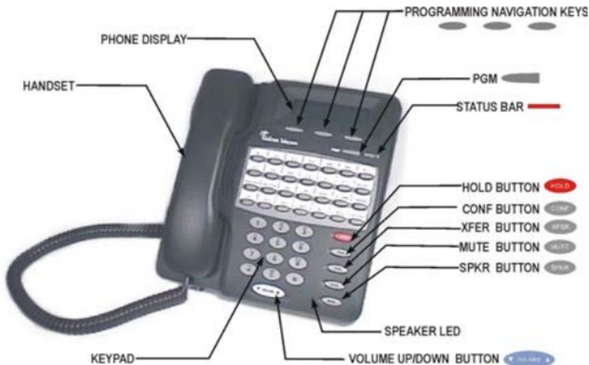
The *Emerald ICE* Standard Model Telephone features a speakerphone, 14 programmable Feature/DSS buttons (dual color LED), Headset Jack, 8 fixed feature keys (Mute, Speaker, Hold, Transfer, Conference, Feature, Volume Up, Volume Down), and one Status Bar type message waiting lamp.
