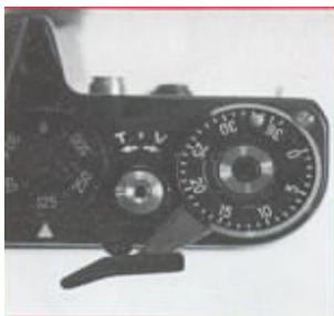
If you do not have a cable release depress the camera's Shutter Release Button until the shutter opens and turn it fully anti-clockwise to the "T" position. The shutter will remain open until the button is returned to the normal position. We recommend the use of a cable release where possible as this will reduce the chance of "camera shake" during the exposure.
