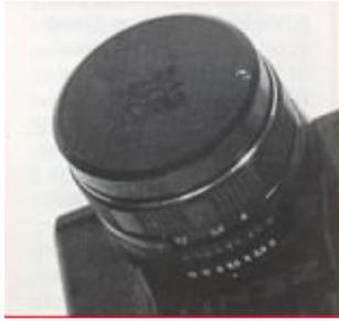
Replace the lens cap to prevent accidental exposure of film during rewinding.
