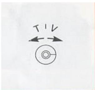
**IMPORTANT**- Do not leave the Shutter Release locked in the "V" position longer than necessary in order to minimize battery drain.
