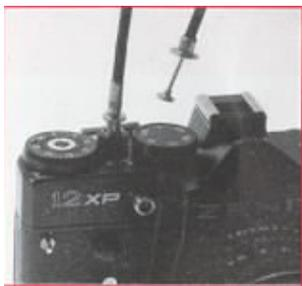
Fit a short cable release (obtainable from any good dealer) into the screwed portion of the camera's Shutter Release Button [3]. Depress the cable release and the shutter will stay open until pressure is released. Some cable releases have a screw lock which avoids the need for holding it during a lengthy exposure.
