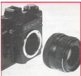
The Zenith lens has a 42mm screw mount and may be removed from the camera body by grasping the whole lens barrel and turning it anticlockwise. Other 42mm screw lenses of a different focal length may then be fitted providing they are of the *single-pin* operating type.
