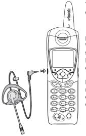
small rubber flap) on the cordless Handset. The plug should fit securely. Do not force the connection.
