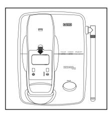
Place a battery pack in the Spare Battery charger. Make sure the metal charging contacts on the underside of the battery pack are aligned with the charging contacts in the Spare Battery charger.
