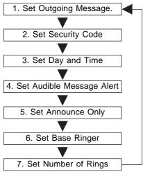
During Answering System setup, the display will flash " -- ". If no key is pressed for 20 seconds, the Answering System will beep, and exit program mode. You can also exit program mode at any time by pressing any **MAILBOX**) key.
