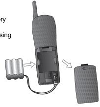
c) Place battery pack in compartment with the wires in the lower left corner, along the bottom of the battery pack.
