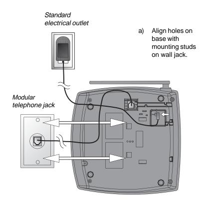
b) Pull base down on mounting studs until it locks into place.
