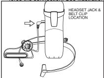
The VTECH VT 9151/VT 9155 is also equipped with a detachable belt clip. Align the pins on the inside edge of the belt clip with the notches on the side of the VTECH VT 9151/VT 9155 handset. The belt clip should snap securely into place. Do not force the connection. See illustration.
