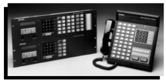
● Telephone Consoles - Currently, two 5.25" high x 19" wide rack or panel mount Telephone Consoles are available. The Model 3110R comes equipped with 9 line keys and the Model 3130R comes equipped with 29 line keys. Both models may be field expanded in increments of 10 lines for a maximum capacity of 99 lines each. The Model 3140D, a desktop telephone console equipped with 39 line keys (non-expandable), is also available.
