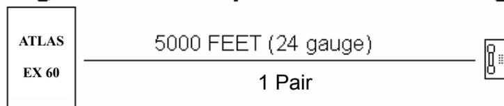
Figure 12: Single Line Telephone cable length
