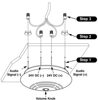
Set volume to maximum (1) before installation and adjust as needed
