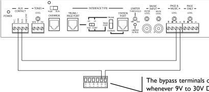
The bypass terminals override the volume control setting whenever 9V to 30V DC (at 25mA) is applied to the D+ and D- terminals. See front page for amplifier and speaker connections.
