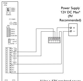
\* Use a 12V regulated power supply. Non-regulated supplies may provide significantly more than 12V when not fully loaded. Greater than 12V supply will cause relay driver to conduct even when not active. A 9V unregulated power supply will typically work appropriately.
