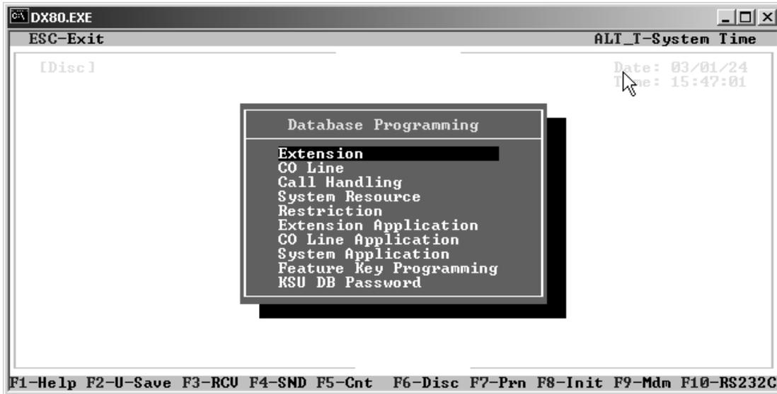
While you are programming the database using PC-DBA programming, the system stores any changes you make in its working directory—not in the DX-80 system memory. When you have finished making your programming changes, you must perform a SEND operation. The system then overwrites the system memory with whatever you have programmed into the working directory. Until you perform the SEND command, **none of your changes are in effect**.
