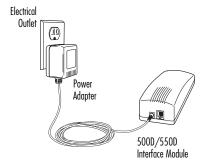
7. Place the SoundStation Premier 500D/550D on a flat, stable surface in the center of the room. If using the extended hypercardiod microphones with the 550D, for the best coverage, position as shown in the examples to the right.
