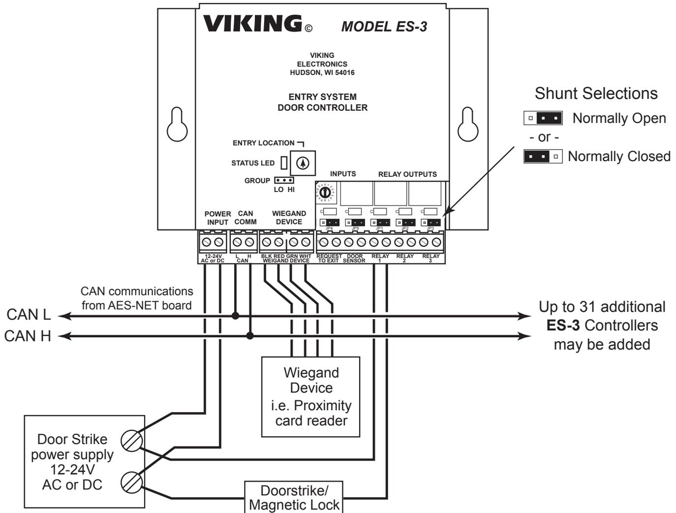
A basic door access controlled entry point is wired as shown above. The **ES-3** may share power with the attached door strike or magnetic lock if the Voltage is between 12-24 Volts and an additional 300 mA of current is available.
