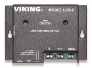
For incoming calls the **LSD-2** can route calls to the **DEVICE 2 (PRIORITY)** port using Caller ID, Distinctive Ring, or Call Back. All other calls will be routed to the phone port. Alternatively, the **LSD-2** can be set up so that all inbound calls are routed to the **DEVICE 2 (PRIORITY)** port. *Note:* Caller ID is not passed through the **LSD-2** to the devices.
