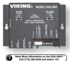
The **DVA-2WA** is a digital announcer with a built in 2 watt amplifier. Designed to provide music and promotion on hold, the **DVA-2WA** can playback in a continuous loop or alternate between promotions and an auxiliary music source in timed intervals. Any number of multiple messages may be recorded. The announcer comes with four professionally pre-recorded promotion on hold messages, a power supply and cabling for an easy plug and play installation.
