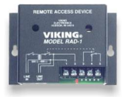
access to system features or an external device. For "line extender" applications, the user does not have to hang up and redial the **RAD-1** to make another call. The **RAD-1** will also provide a hookswitch flash on the **LINE OUT** port to access PABX, Centrex or Electronic Key system features.
