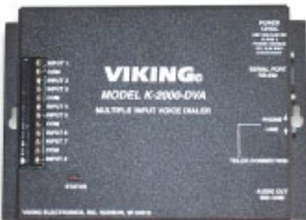
Viking's **K-2000-DVA** is a fully programmable multi-input, multinumber auto dialer and digital announcer, designed for emergency and non-emergency message notification. The **K-2000-DVA** has eight dry contact inputs which when tripped will sequentially dial up to 8 different phone numbers and play a recorded message corresponding to the input tripped.
