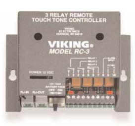
The **RC-3** enables a standard Touch Tone phone to control up to 3 maintained ON, maintained OFF, or momentary relay contacts from a remote location. The **RC-3** is fully user programmable and uses non-volatile E<sup>2</sup> memory.
