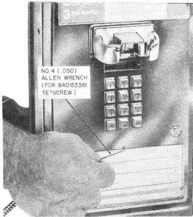
**FIG. 1 - Loosening or Securing Instruction Cards
