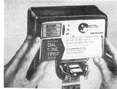
**FIG. 2 - Installing Instruction Cards (All 1-Type and
