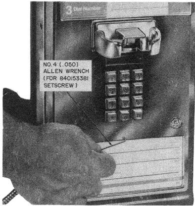
Fig. 21—Securing Instruction Card (Typical)
