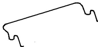
FIG. 1 - 840157333 Trap Lever Spring
