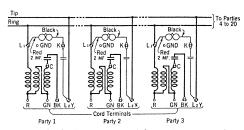
Fig. 1—Bridged Ringing Anti-Sidetone Stations—High Impedance Ringers
